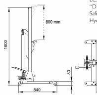
LCS lowering contro system. "Dead man`s" principle operation. Safety overload valve. Hydraulic stroke limitation.
